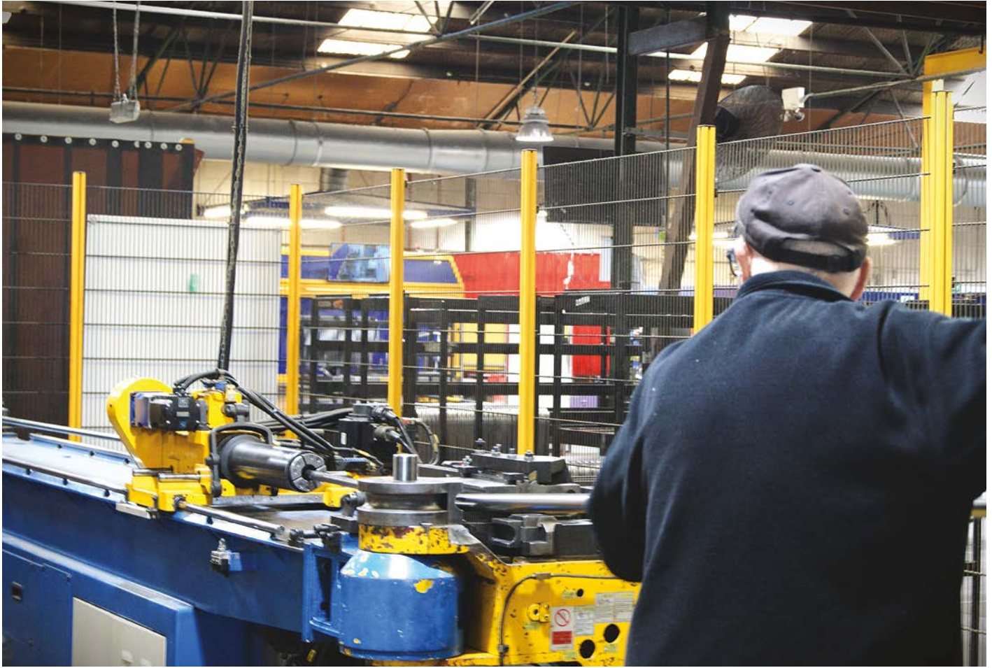
Phil feeds the steel tubes into the machine and out come perfect legs for chairs and tables
